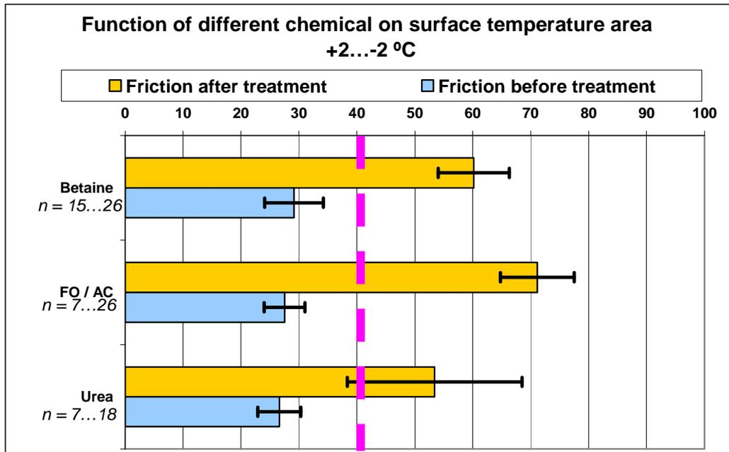
Figure 5 – Friction levels with 95 % confidence intervals of different chemicals when anti-skid treatment is being performed. Friction requirement of the runway is 40 in Finland. [4]
