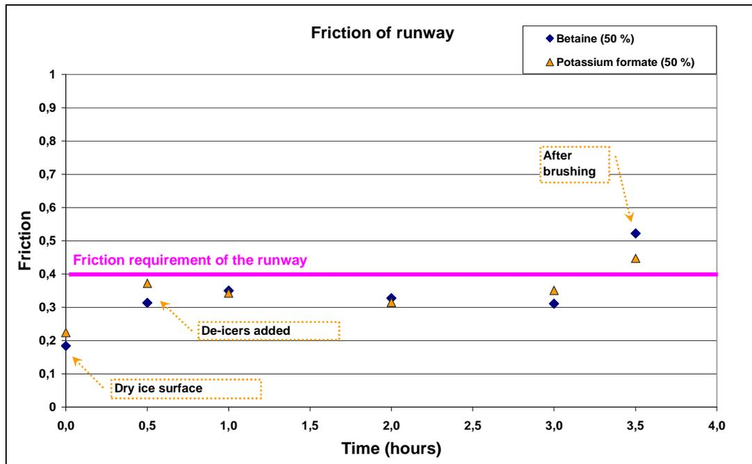
Figure 3 - Friction test results. The effect of brushing on friction is clearly visible in the results. However, no differences between these agents were recognized; both chemicals passed the requirement. [3]
