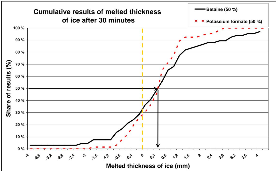
Figure 2 - Cumulative results of field tests measuring de-icing efficiency of different agents. No deviations were found in the efficiencies of these agents. [3]
