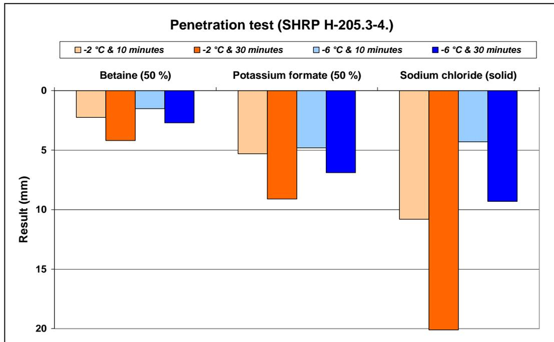
Figure 1 - Results of the penetration test made on betaine, potassium formate and sodium chloride.[1] [2]
