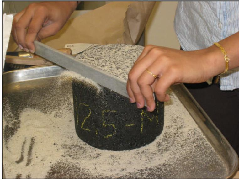
**FIGURE 2 – Modified Sand Patch Test**
