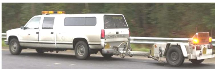
**Figure 2 The pavement friction tester**
