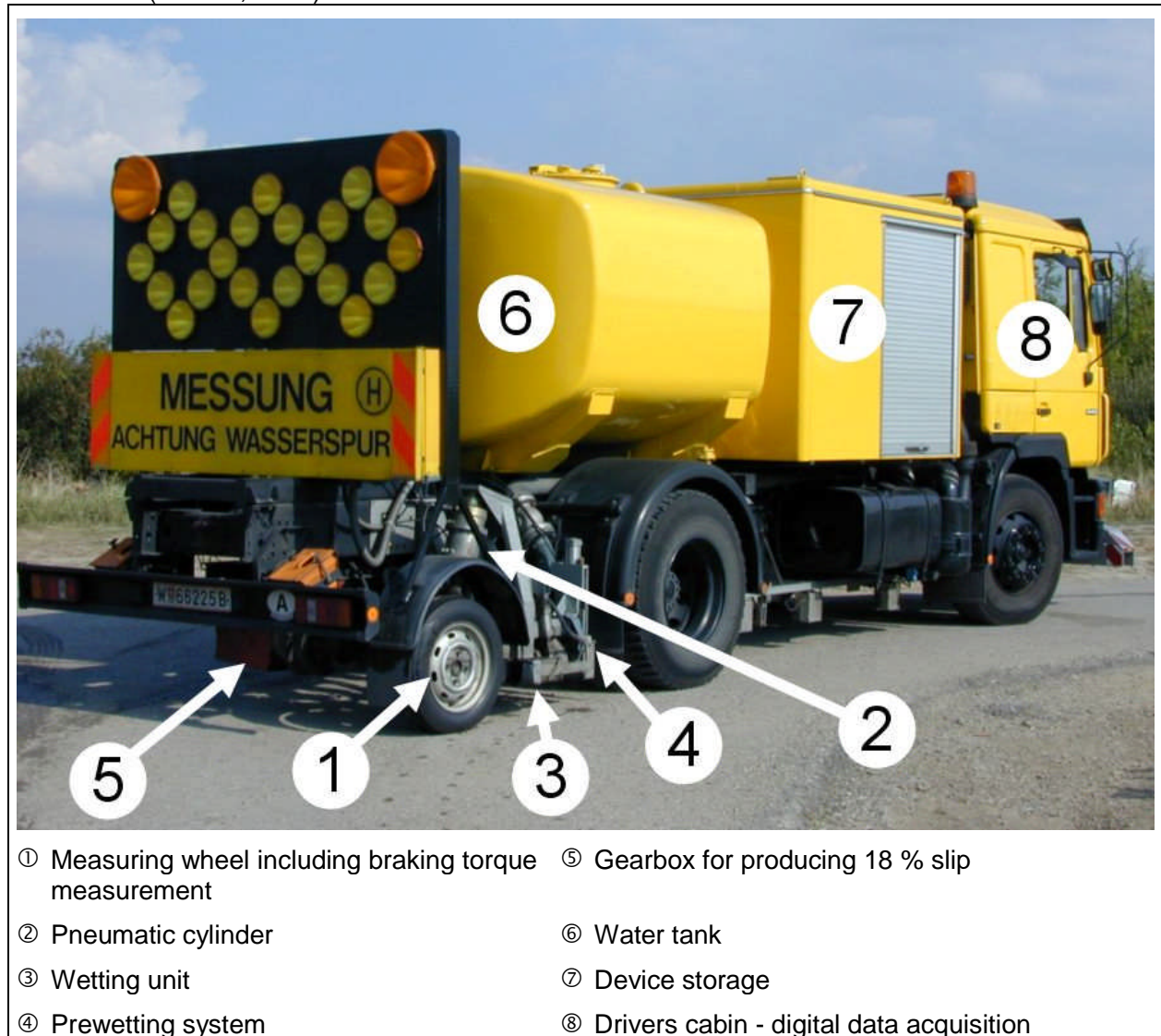
Figure 1: RoadSTAR (Road Surface Tester of arsenal research)
