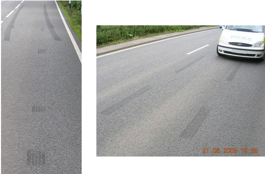
Figure 2 - Left: ABS “dashes” observed on an NTS in Dorset following ABS testing (No ABS skid marks in background) Right: Semi continuous ABS “dashes” observed on an NTS in Derbyshire following testing
