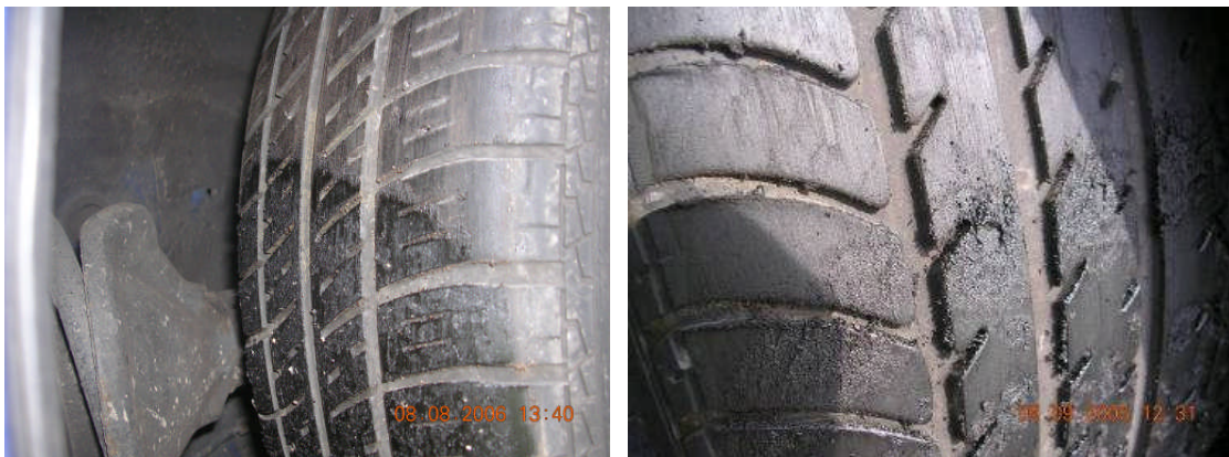
Figure 3 - Left: Oily deposit observed following No ABS test on SMA in Devon, Right: Oily deposit and bitumen observed following No ABS test on SMA in Dorset
