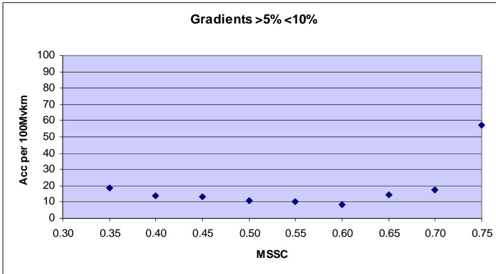
The sites that are greater than an MSSC of 0.65 have been removed and the graph redrawn and is shown in Figure 5.
