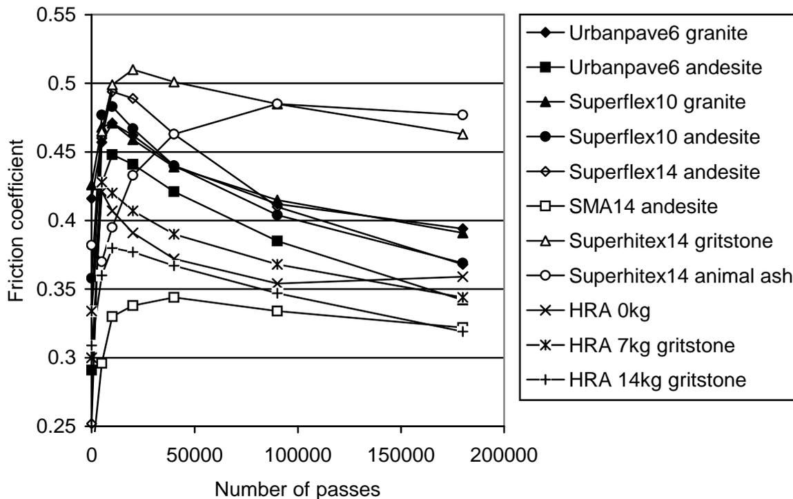
Figure 1 Average WS friction coefficient
