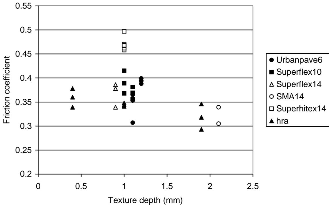
Figure 4 Plot of WS for the asphalt mix against texture depth in relation to mix type
