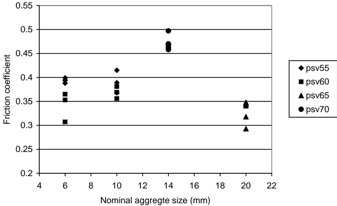
Figure 3 Plot of WS for the asphalt mix against nominal aggregate size in relation to PSV
