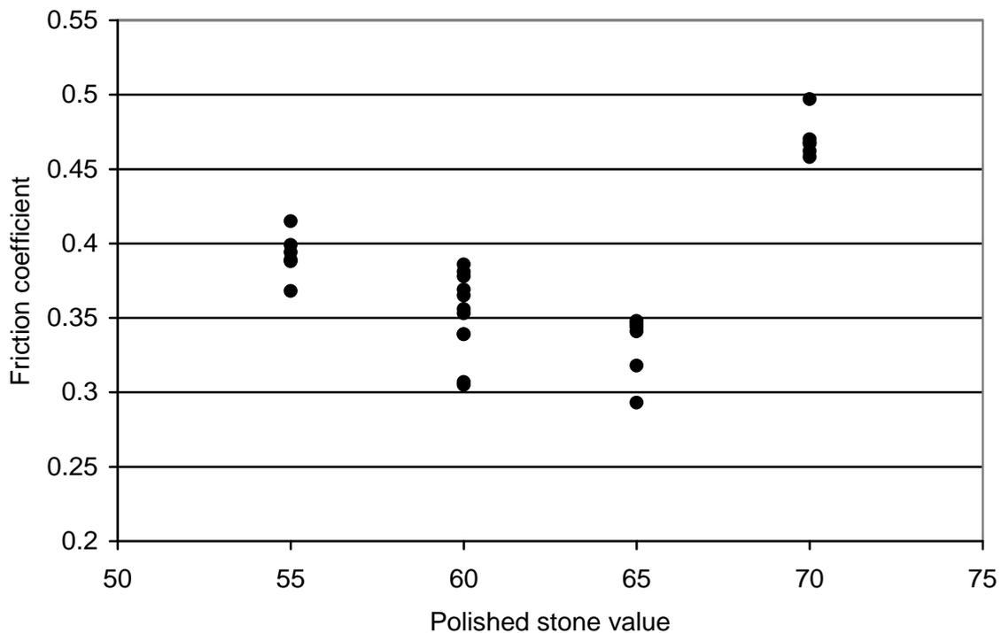
Figure 2 Plot of WS for the asphalt mix against PSV of the aggregate used
