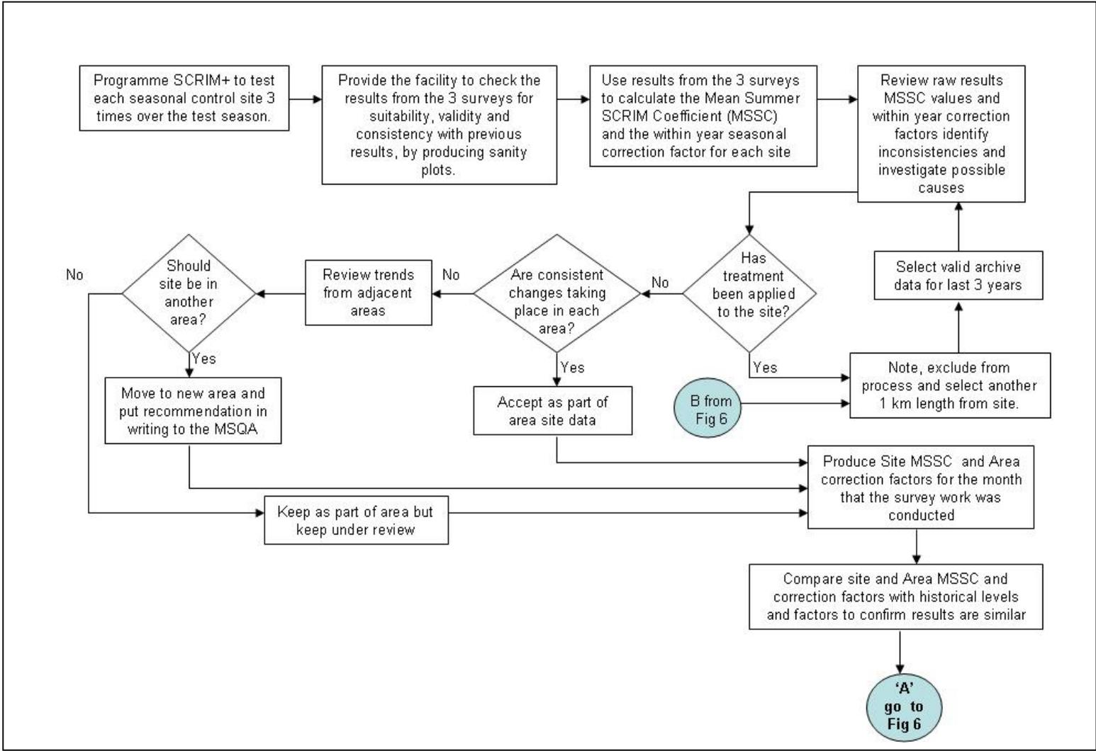
**Figure 6. Process diagram showing the production of MSSC and ESC and their respective correction factors for New Zealand, Part 2**
