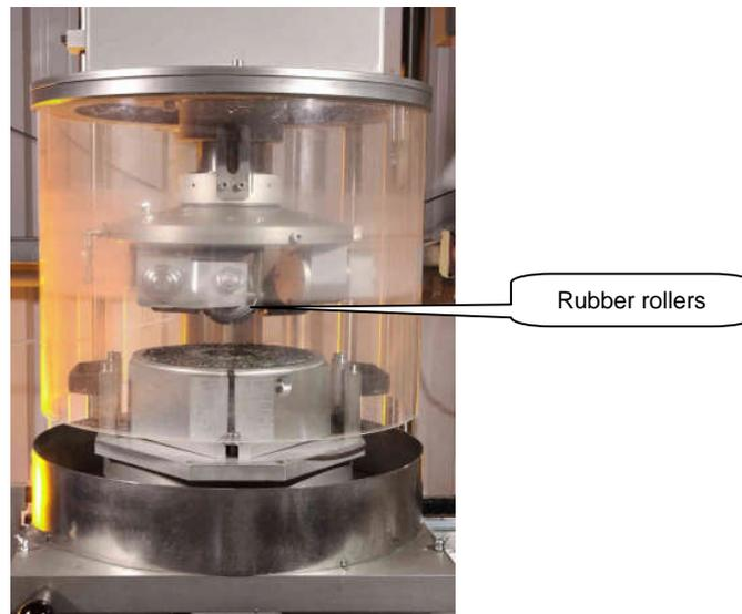
**Figure 1.2 Specimen in polishing mode**
