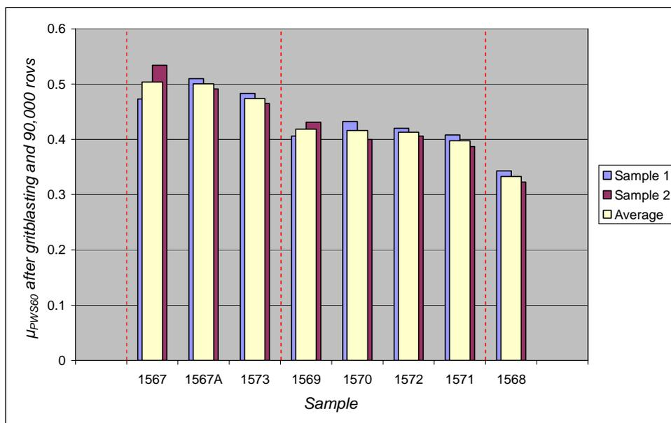
Figure 2.1 Results of Stage 1  $\mu_{PWS\ 60}$  measurements
